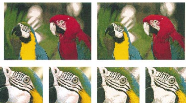
Fig. 8. At the top from left to right: Parrots 16 colors (a) FLS; (b) N -convex. Illustration of the error type produce by FLS and N -convex method. The detailed images, from left right: (a) FLS, K = 256 ; (b) N -convex; K = 256 ; (c) FLS, K = 16 ; and (d) N -convex, K = 16 .
