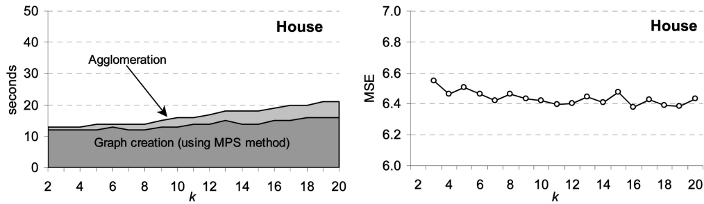
Fig. 5. The running time and the quality of the DLA as functions of k .
