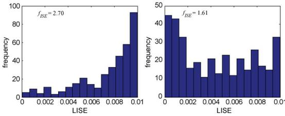
Fig. 10. LISE distribution of all the approximated edges with  $\varepsilon = 0.01$  for Curve II. The best approximation result (right) with  $f_{ISE}(P') = 1.61$  is found from all the *equivalent solutions*, which is much lower than result after Algorithm II (left) with  $f_{ISE}(P') = 2.70$ . Both approximation results have  $M = 364$ .
