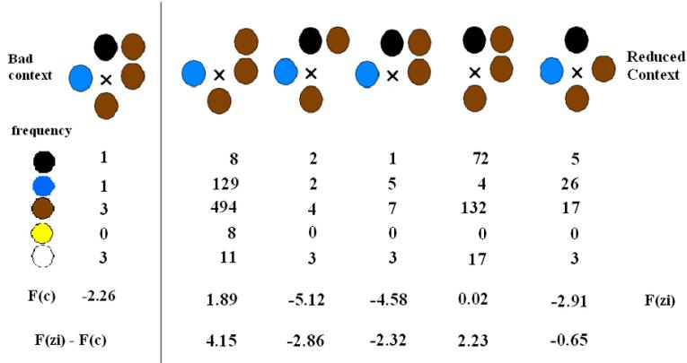
*Fig. 2.8 Bad context and its reduced context, black pixel is possible a noisy pixel with high  $F(z_i) - F(c)$  difference*
