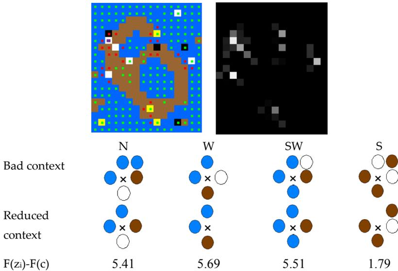
*Fig. 2.9 Sample image with good and bad context demonstrated in red and green colors (top left), its voting image (top right). Voting example for the white pixel labeled with purple with accumulated  $F(z_i) - F(c)$  value 18.30 (bottom).*
