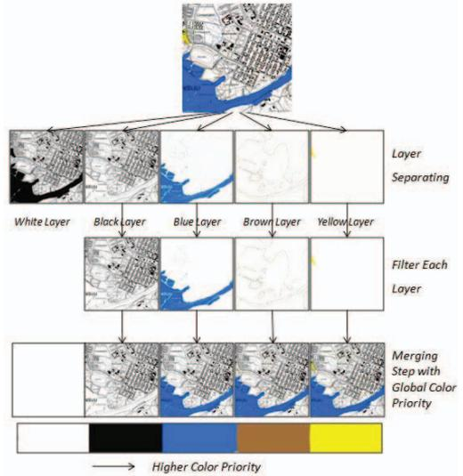
Fig. 1 Multi-layer framework using global layer ordering
