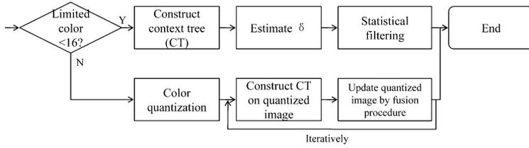
Fig. 12. Workflow of the proposed adaptive context-based method.
