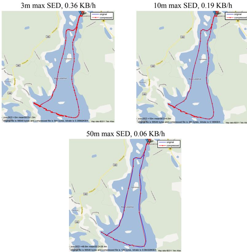
**Fig. 5.2.** Compression example of the proposed GPS trajectory compression (GTC) algorithm.
