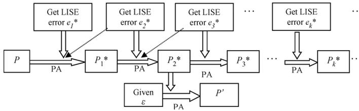
Fig. 12. Workflow of the proposed bottom-up multiresolution method. Error tolerance of coarser resolution is selected as high threshold for polygonal approximation, which is labeled by dashed line in the figure. In this example, if  $e_2^* < \varepsilon < e_3^*$ , then the approximation of  $P_3^*$  and  $P_4^*, \dots$  can be skipped.
