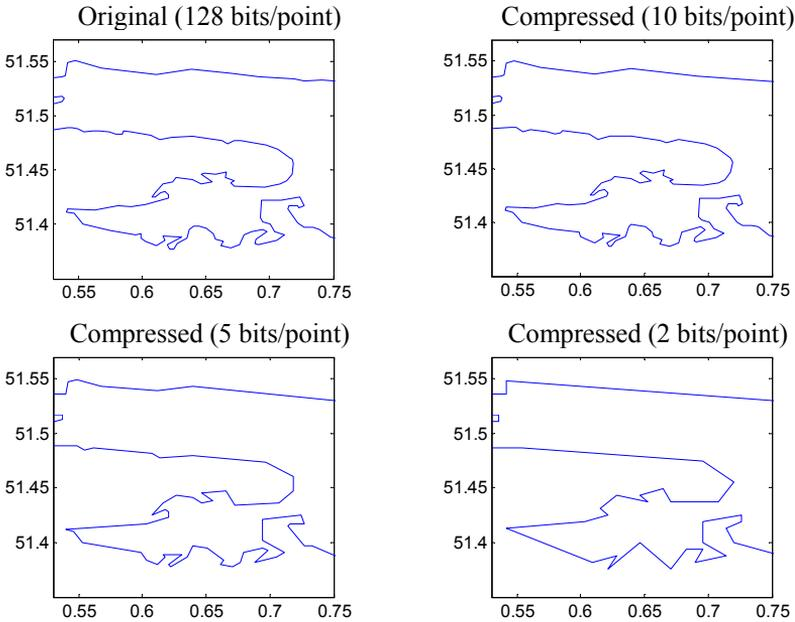
Fig. 4.4. Performance under different bit-rate on a fragment of the testing UK map with 10911 points.
