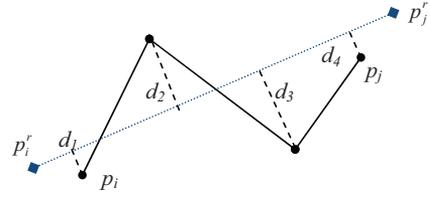
Fig. 2, Poly-line  $\{p_i, \dots, p_j\}$  (solid line) is approximated by  $\{p_i^r, p_j^r\}$
