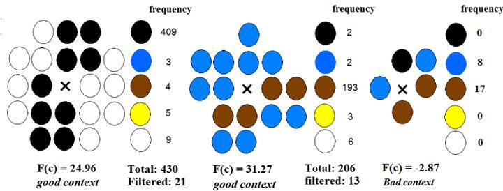
Fig. 2.4. Examples of context distribution: the pixels in the left and middle contexts are filtered using the dominant color, whereas no filtering is done for the pixel in the context on the right.
