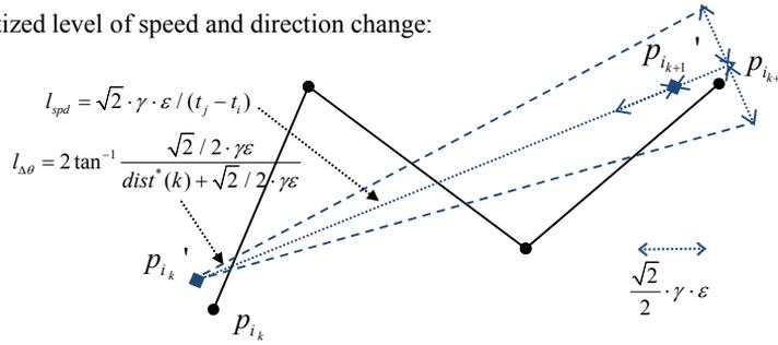
**Fig. 5.1.** An example of the quantization process for the GPS trajectory
