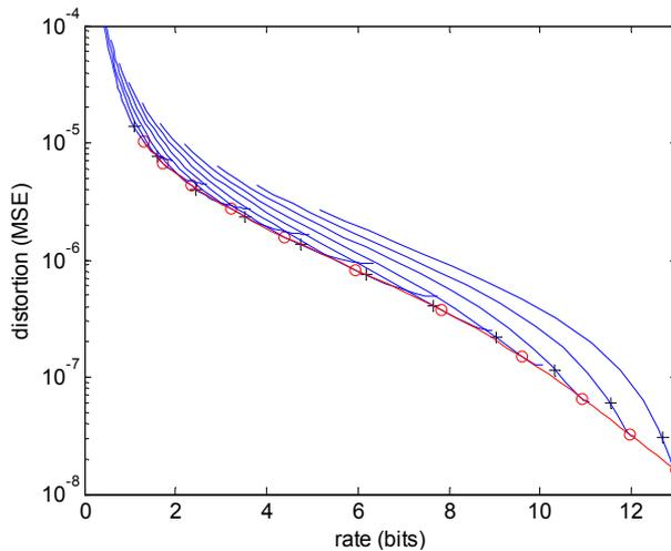
**Fig. 4.3.** Rate-distortion curve for quantization step  $q_k=0.01/2^k$ , where  $k = 0, 1/2, 1, \dots, 5$  (from left to right), black '+' is the position when error balance principle is applied, red 'o' is the proposed. The red line is the rate-distortion curve when optimal  $\lambda$  is selected.
