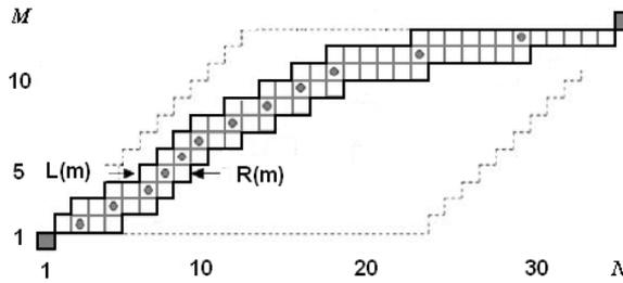
**Fig. 3.2.** An example of the reduced search dynamic programming with  $N = 35$  and  $M = 14$ , where the width of the bounding corridor  $W = 2$ . Reference curve is represented with the gray circles while the full state space is surrounded by the dashed line.
