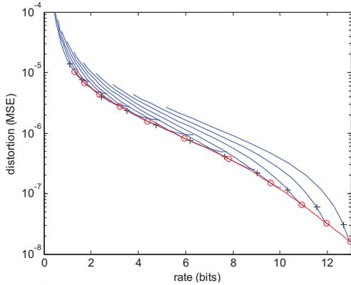
**Fig. 3.** Rate-distortion curve for quantization step  $q_k=0.01/2^k$ , where  $k=0, 1/2, 1, \dots, 5$  (from left to right), black '+' is the position when error balance principle is applied, red 'o' is the proposed ( $\lambda$  is selected by (10)). The red line is the rate-distortion curve when optimal  $\lambda$  is selected with  $q_k=0.01/2^k$ , where  $k=0, 1/5, 2/5, \dots, 5$ .
