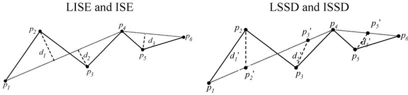
Fig. 1. Example of calculating ISE, LISE, LSSD, and ISSD. Given  $P = (p_1, p_2, p_3, p_4, p_5, p_6)$  and the approximated curve  $P' = (p_1, p_4, p_6)$ , where  $p_2', p_3',$  and  $p_5'$  are the approximated temporally synchronized position. (Left) ISE is estimated as  $d_1^2 + d_2^2 + d_3^2$ , and LISE is estimated as  $d_1^2 + d_2^2$ . Meanwhile, (Right) ISSD is estimated as  $d_1'^2 + d_2'^2 + d_3'^2$ , and LSSD is estimated as  $d_1'^2 + d_2'^2$ .
