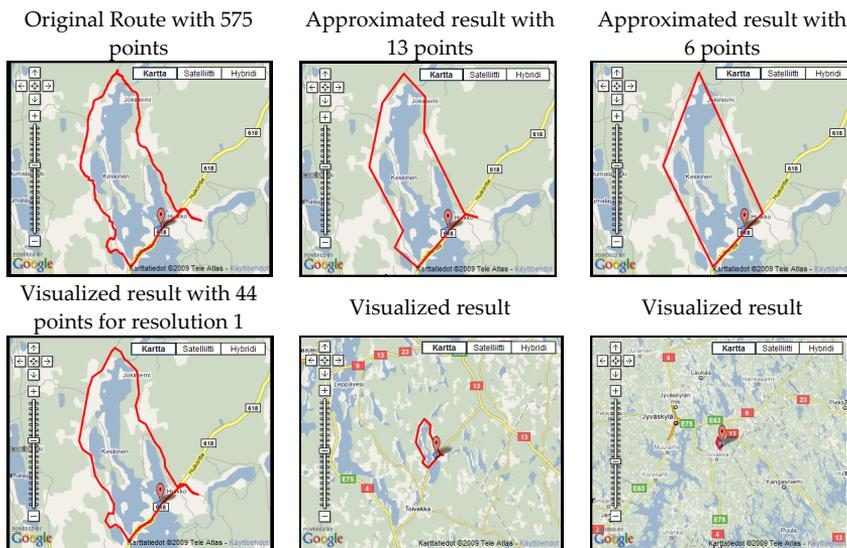
*Fig. 3.7. Example of the GPS trajectory simplification by the proposed algorithm.*
