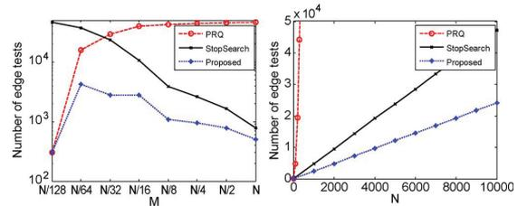
Fig. 2. Number of *edges tests* for solving the *min-# problem* (left) under different error tolerance and (right) with different number of input vertices for U.K. map (Curve II). In the left figure, the resulting number of output vertices  $M$  is shown in the  $x$ -axis instead of the given error tolerance.
