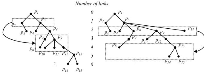
Fig. 5. Example of reducing the number of output vertices with a width of bounding corridor  $W = 2$ : (left) the target vertices with one link and (right) the target vertices with two links after tree structure updated given  $\delta(P_3^9) < \varepsilon$ ,  $\delta(P_3^{11}) < \varepsilon$ . (Left figure) Typical example after the initialization step for Algorithm I.
