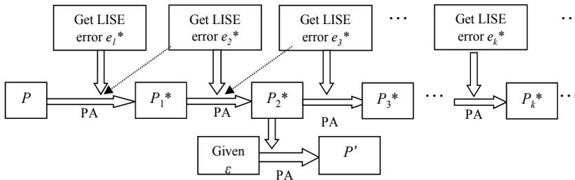
**Fig. 3.6.** Workflow of the proposed bottom-up multi-resolution method. Error tolerance of coarser resolution is selected as high threshold for polygonal approximation, which is labeled by dashed line in the figure. In this example, with  $e_2^* < \epsilon < e_3^*$  the approximation of  $P_3^*$  and  $P_4^*$ ,... can be skipped.
