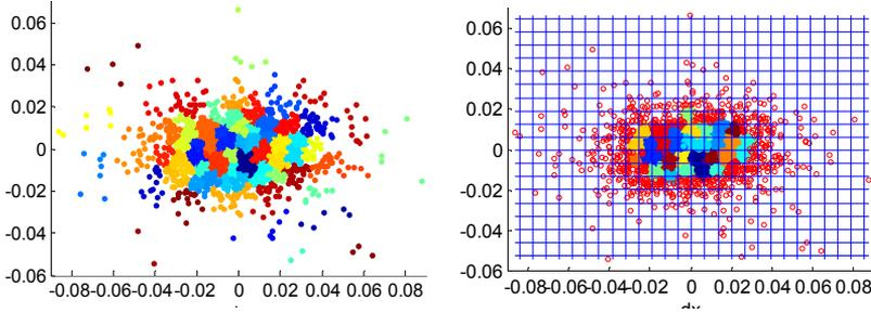
**Fig. 4.5.** Demonstration of the outlier selection (5 bits/point constraint). ECPNN with  $MSE=8.7 \cdot 10^{-6}$  and codebook size 78 (left). The proposed two-level codebook with  $MSE=6.9 \cdot 10^{-6}$  and size 30 (right). Outliers are marked as 'o'. Grid size for uniform quantization is also labeled. The testing curve is the UK map with 10911 points.
