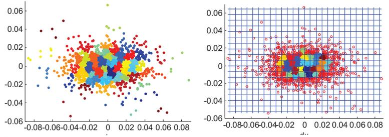
**Fig. 3,** Demonstration of the outlier selection (5 bits/point constraint). ECPNN with MSE=  $8.7 \cdot 10^{-6}$  and codebook size 78(left). The proposed two-level codebook with MSE=  $6.9 \cdot 10^{-6}$  and size 30 (right). Outliers are marked as 'o'. Grid size for uniform quantization is also labeled.
