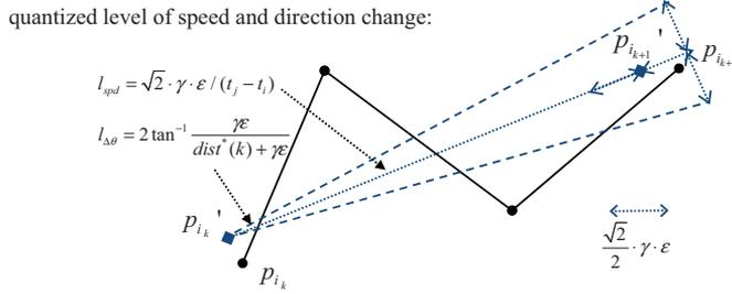
**Fig. 1:** An example of the quantization process for the GPS trajectory
