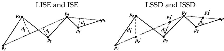
**Fig. 3.1.** An example of calculating ISE, LISE, LSSD and ISSD. Given  $P = (p_1, p_2, p_3, p_4, p_5, p_6)$ , and the approximated curve  $P' = (p_1, p_4, p_6)$ , where  $p_2'$ ,  $p_3'$  and  $p_5'$  are the approximated temporally synchronized position. ISE is estimated as  $d_1^2 + d_2^2 + d_3^2$  and LISE is estimated as  $d_1^2 + d_2^2$  (left). Meanwhile, ISSD is estimated as  $d_1^2 + d_2^2 + d_3^2$  and LSSD is estimated as  $d_1'^2 + d_2'^2$  (right).
