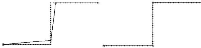
**Fig. 3.4.** An example of equivalent solutions in min-# approximation, where both approximated curves meet the error tolerance  $\epsilon = 2$  and have same output  $M = 4$ .
