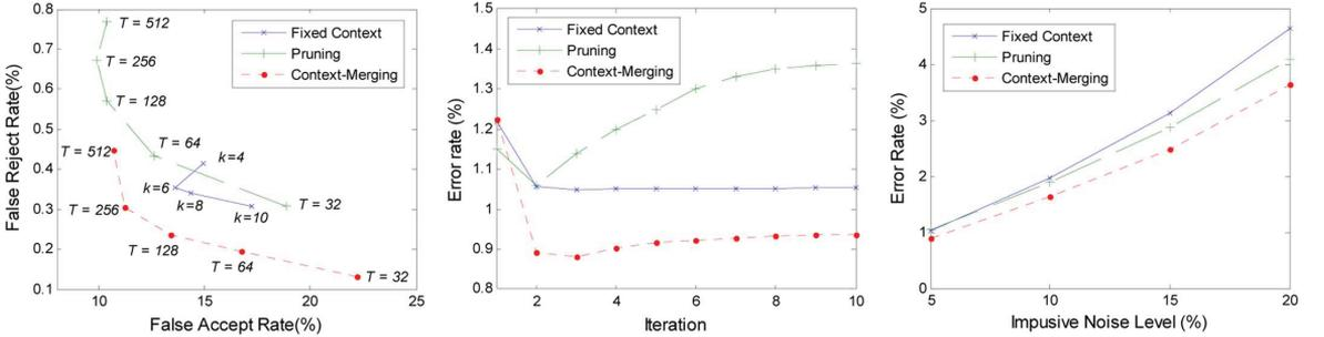
Fig. 6. *False acceptance rate* (FA), *false rejection rate* (FR), and *error rate* are evaluated on different conditional probability estimation algorithms for filtering impulsive noise. The performances are compared by selecting different thresholds  $T$  (left), different iterations (middle), and different noise levels (right). Image #2-05 is used as the test image by adding 5% impulsive noise (left and middle), while  $T = 128$  and  $k = 8$  are used in the middle and on the right.
