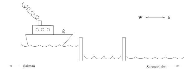
12. Construct a lock automaton for a channel, which opens and closes the locks and increases and decreases the water level automatically. The Western lock gate can be opened only when the water is up and the Eastern gate only when the water is down. You can control the water level only when both gates are closed. The automaton gets the following input data from the control system:
