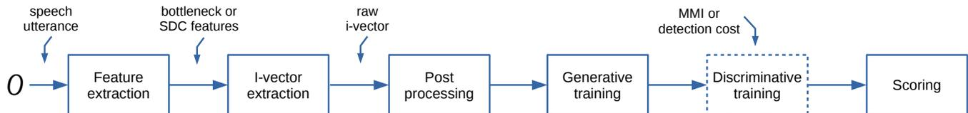
Fig. 3. Block diagram of our language detection system. We use bottleneck features for LRE’15 and shifted delta cepstra features for I2R Dev, while all back-end preprocessing and classifiers for i-vectors are the same.
