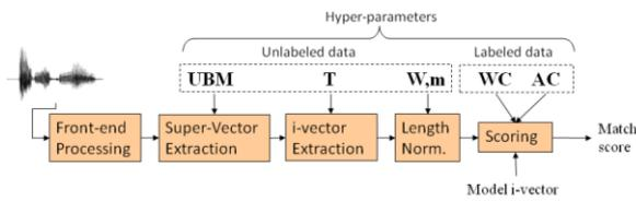
Figure 1: Simplified block diagram of i-vector extraction and scoring.
