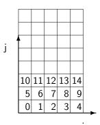
Key point is that in final read, each thread in the warp is reading from a different shared memory bank – there are 32 of these.
