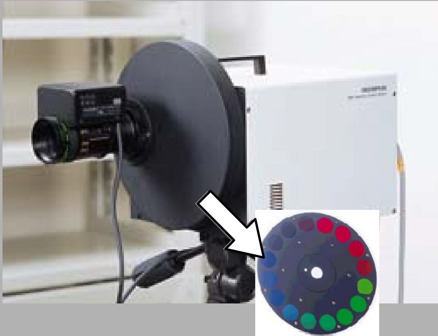
16-band multispectral camera for still image
