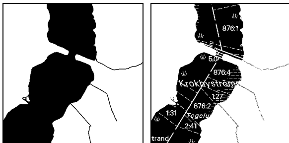
Figure 6: The original water layer (left), and the same information when obtained by color separation (right).
